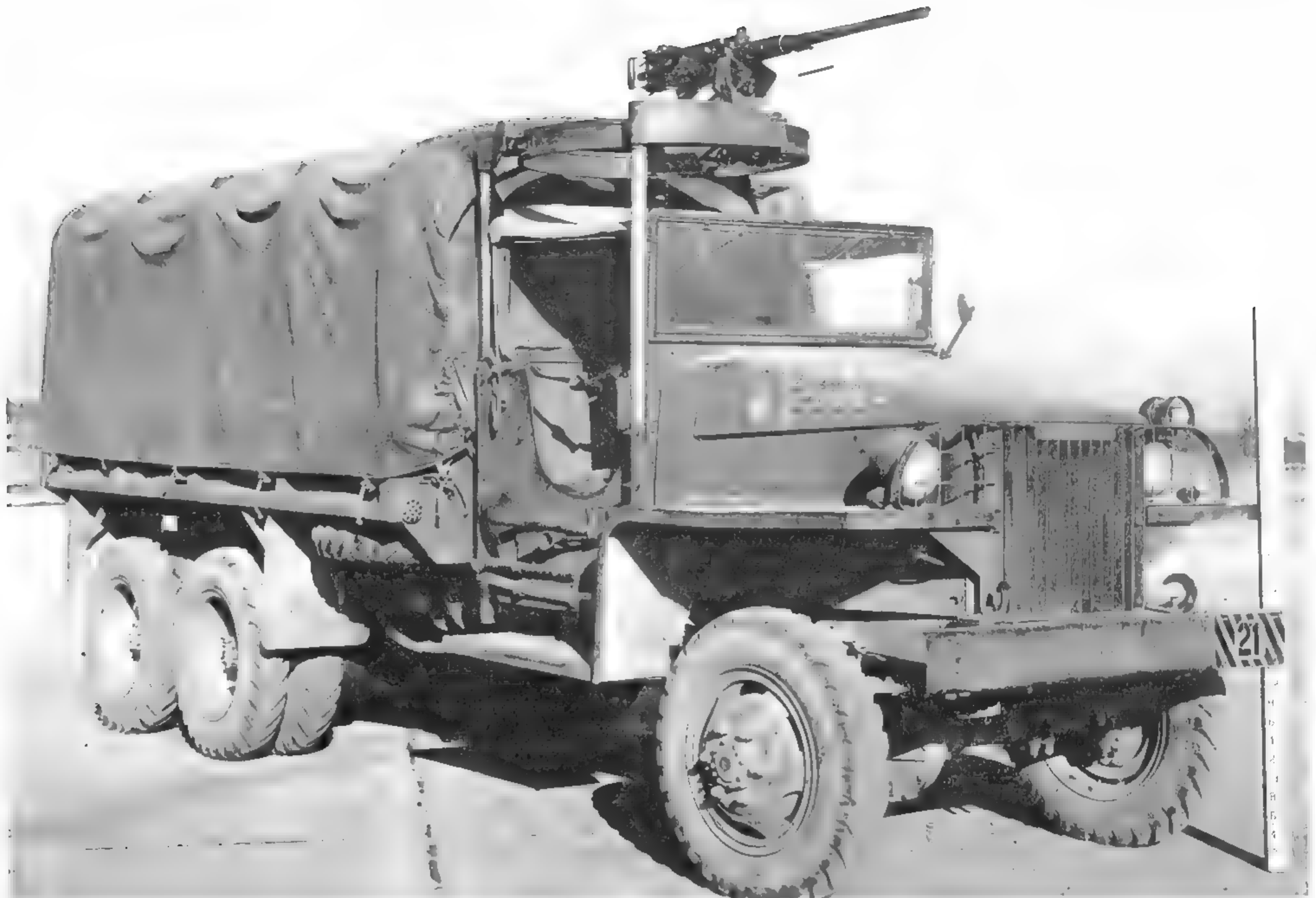
The M36 mount was the most common ring mount used during WWII. It could be installed on all the open-cab 6x6 trucks the U.S. Army fielded during WWII, including the DUKW. This November 1943 photo shows an early prototype of that mount installed on the vehicle that pioneered the military standard open cab — the rare open-cab US6 Studebaker. (U.S. Army photo)
